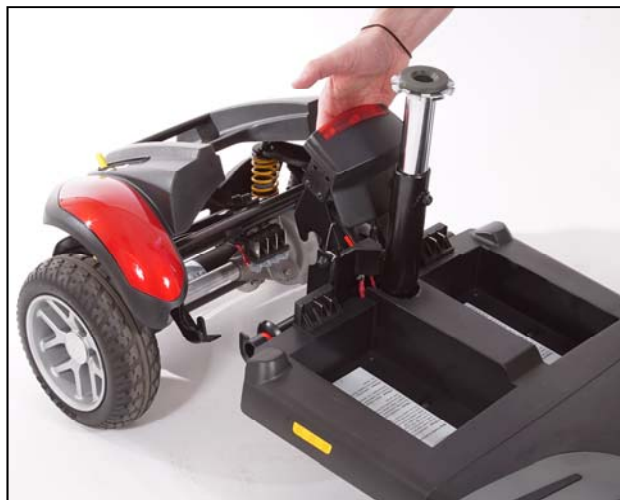
Figure 19. Separating the Drivetrain and Frame
