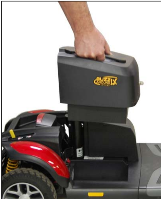
Figure 23. Battery Pack Installation
