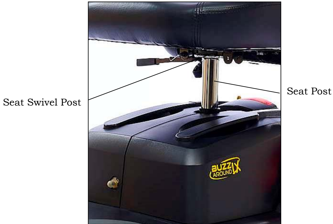
Figure 25. Installing the Seat
