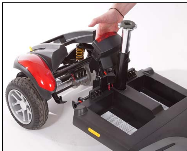
Figure 17. Separating the Drivetrain and Frame
